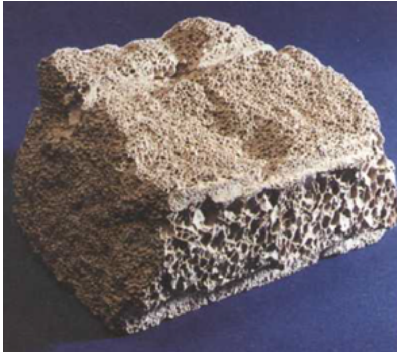
Reinforced Autoclaved Aerated Concrete (RAAC)
